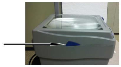
• Removing the old bulb. There may or may not be a cover over the bulb. If there is, open the cover by simply lifting up on the tabs identified in the picture below.
