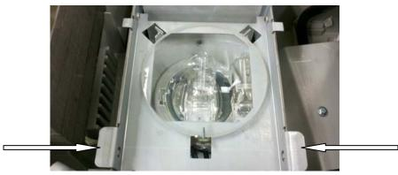
• When the cover is open, pull the bulb out of the socket. (They can be somewhat difficult to pull out and may require a firm pull.) As you saw in the picture of the bulbs earlier in this handout, they are attached by two prongs.
